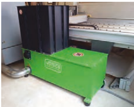
Top: Crusher EZ 6/1 apart from a plate cutting saw for shredding remains of chip board and multiplex panels
