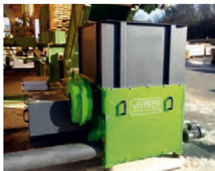
Left: EZ 10/2 , Power 37 KW, Filling with scrap wood via the conveyor belt, material discharge via a screw to the slate floor conveyor.
