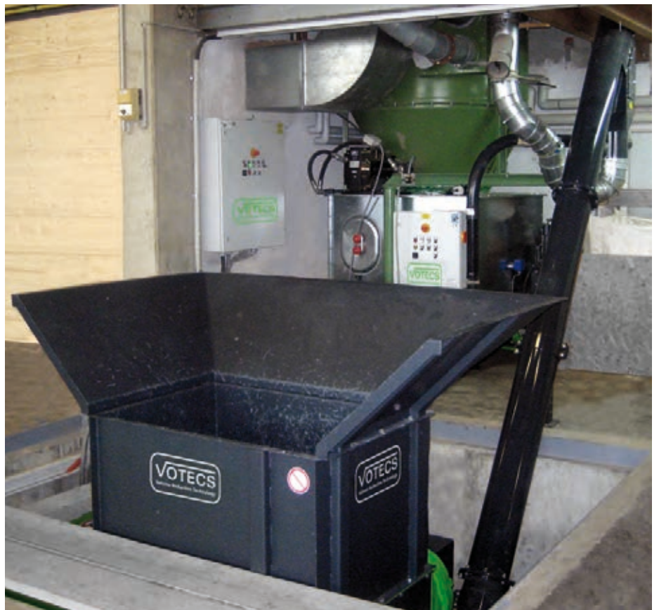
Left: EZ 13/2 with a discharge screw conveyor on a platform to transport the materials to the conveyor belt.
