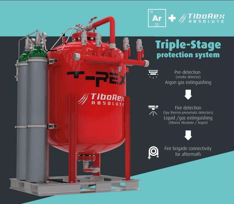
**In the first stage,** in the first phase, there is an alarm via smoke detectors. This detection activates the Argon gas extinguishing system. In this way there is a prior deprivation of oxygen inside the container, removing the strength of the fire and avoiding explosions.
