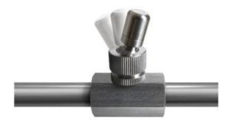
The three FINESTFOG high-pressure nozzles were specially developed to guarantee optimal humidity distribution with finest atomization without the need for support by a carrier gas. The nozzle achieves the finest atomization at a water pressure of approx. 80 bar.
